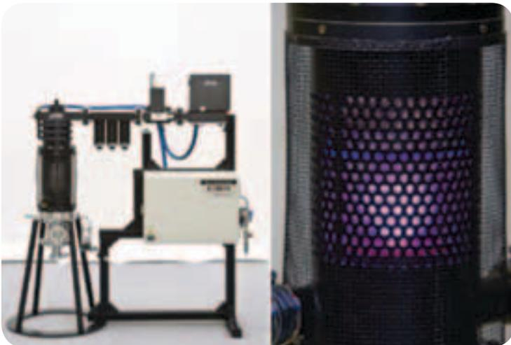
*The diamond plasma chemical vapor deposition system to be installed at Ohio State will enable the synthesis of diamond electronic devices.*
