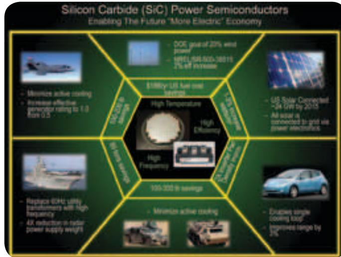
The substance can be used in power semiconductors that operate at higher temperatures, higher switching frequencies and lower switching losses for engine starting, emergency power, battery charging and circuit breakers.
