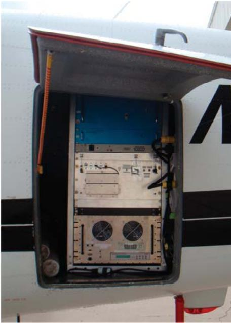
*Figure 1. Photo of OSU sensor (lower component in rack) in Twin Otter Aircraft utilized in recent airborne observations.*
