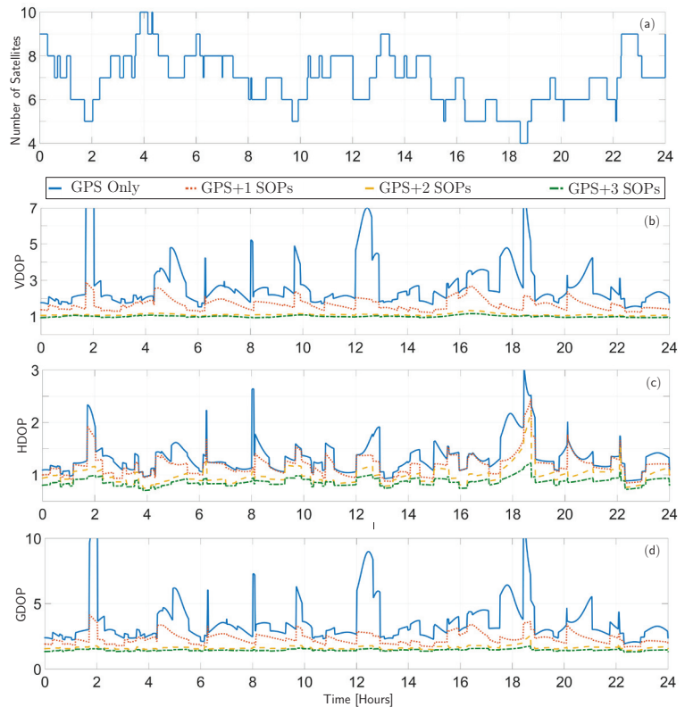
FIGURE 2 Fig. (a) represents the number of SVs with an elevation angle >20^\circ as a function of time. Fig. (b)-(d) correspond to the resulting VDOP, HDOP, and GDOP, respectively, of the navigation solution using GPS only, GPS + 1 SOP, GPS + 2 SOPs, and GPS + 3 SOPs.
