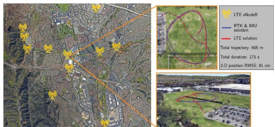
Figure 1. Experimental results with real 4G LTE signals using a non-differential opportunistic navigation framework: environmental layout of the experiment, location of the eNodeBs, ground truth and final navigation solution. Map data: Google Earth.
