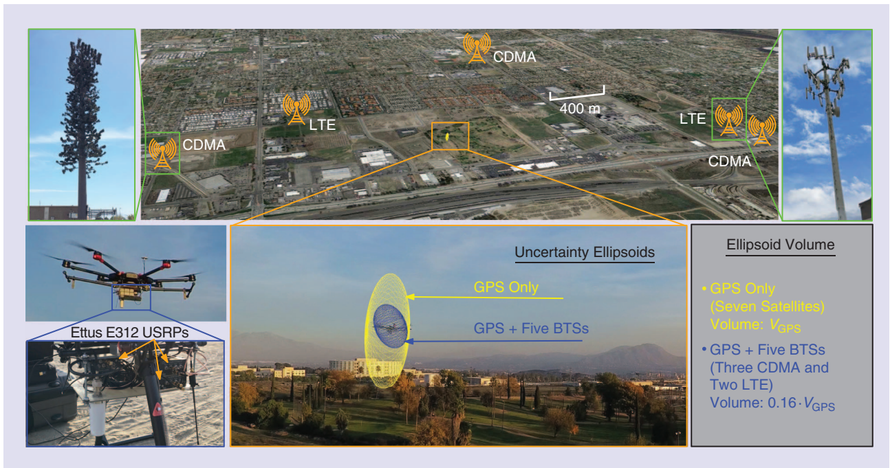
FIGURE 8. Experimental results comparing the navigation solution uncertainty ellipsoids produced by GPS alone and by the multisignal navigation SDR (GPS and cellular CDMA and LTE). (Map data courtesy of Google Earth.)
