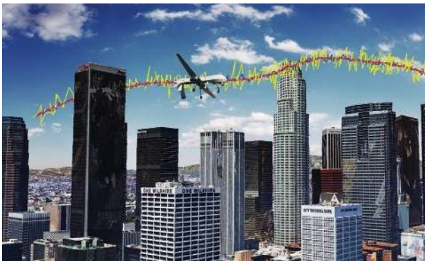
Simulation results for an unmanned drone showing the true trajectory (red) with GPS navigation only (yellow) and GPS aided with cellular signals (blue). Image source: UCR.
