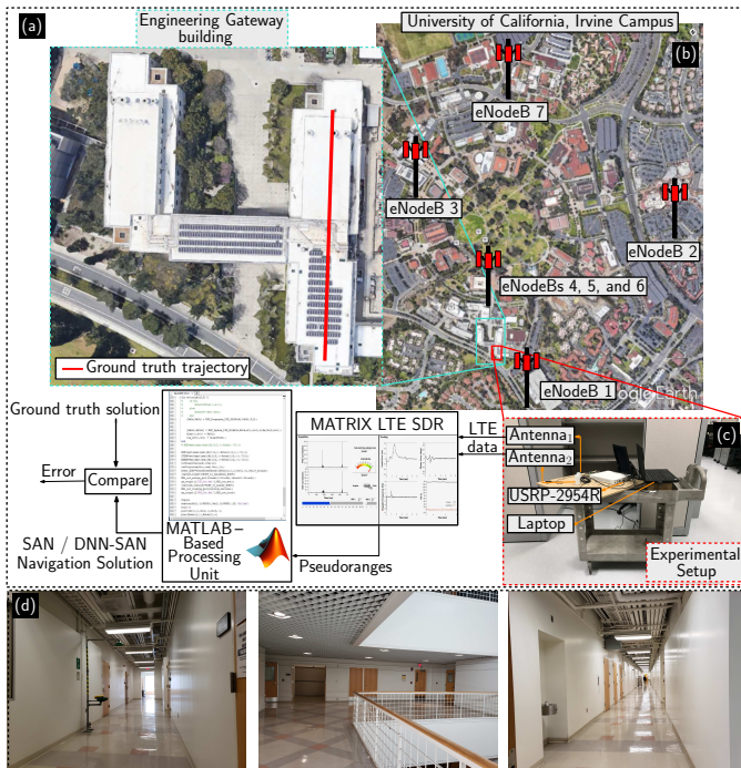
Fig. 8. Environmental layout and experimental setup for experiment 1-a: (a) Engineering Gateway building where the experiment was performed and the ground truth trajectory, (b) LTE eNodeBs' positions, (c) experimental setup, and (d) sample photos of the environment.
