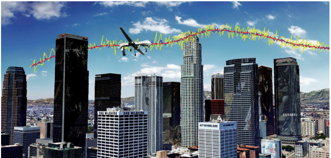
FIGURE 1. The simulation results for an unmanned drone flying over downtown Los Angeles showing the true trajectory (red line) with GPS navigation only (yellow line) and GPS aided with cellular signals (blue line). (Figure used courtesy of UCR.)
